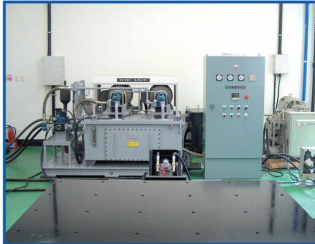
Hydraulic Pump Unit has designed according to vibration tester's characters such as high speed and high frequency. It provide enough discharge rate and stable temperature control.
