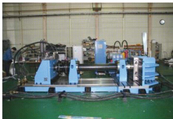
50kN Torsion Fatigue Tester
