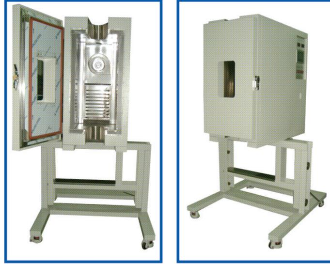
1. This equipment is adhered to tensile strength tester. It can be tested according to choice of temperature, humidity , ultra low temperature or high temperature otherwise it also can be applied to FIRE testing.
