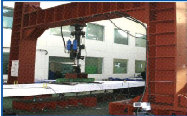
1. Strength test of construction, engineering, other structures with the temporary control volume (load, displacement, strain) by the various waveforms
